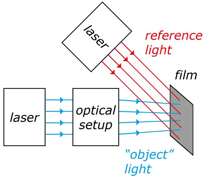
*holographic optical element recording*
